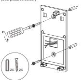
3. After finishing wiring job , put the Main Unit on the hanger and then fix it with the screws to complete the whole installation
