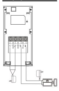
1) The power supply unit is AC/DC 8~36V 2) Please choose the power supply for unlocking according to the requirement.
