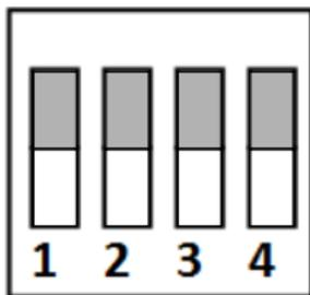
Figure 2. 1 DIP Switch Module (Binary Code: 0000)
