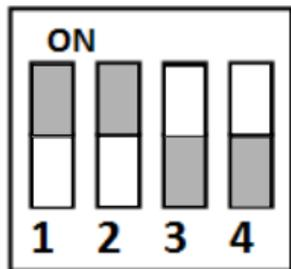
Figure 2. 2 DIP Switch Module (Binary Code: 0011)
