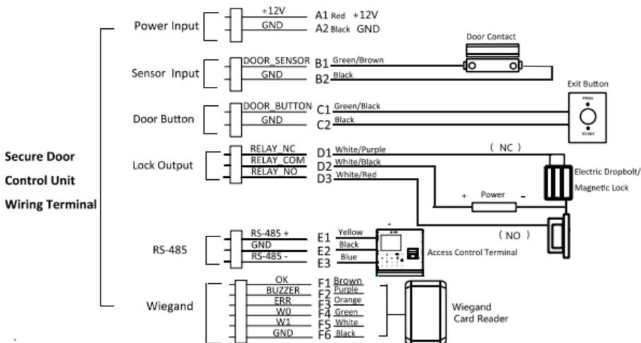
Figure 3. 1 External Device Wiring
