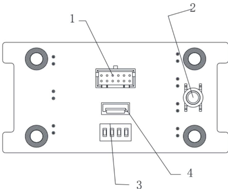
Figure 1. 2 Rear View of Secure Door Control Unit
